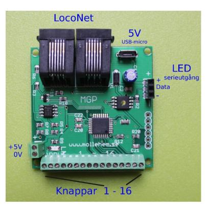
LEDs are connected though drivers and the drivers are connected to the decoder in series through a serial bus. The serial bus uses normal extensions cables type R/C servo extensions.
